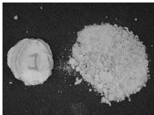
Figure 3 The stone samples after testing. The sample on the left was tested at a strain rate of 0.0002 \text{ s}^{-1} . Part of the sample flaked off after testing as a result of handling. The powder on the right was produced during a high strain rate test.
